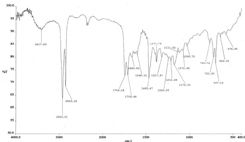
**Figure 9 IR spectrum of CK<sub>2</sub>**
