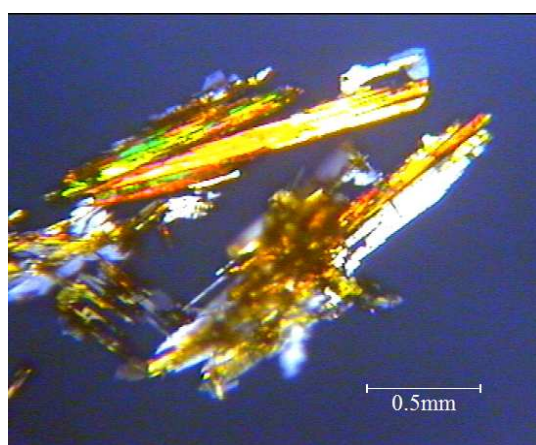
Figure 2. The polarimetric images of Ph 4 P[CrO 3 Cl], method: slow evaporation, solvent: CH 2 Cl 2 , Temperature:0°C.
