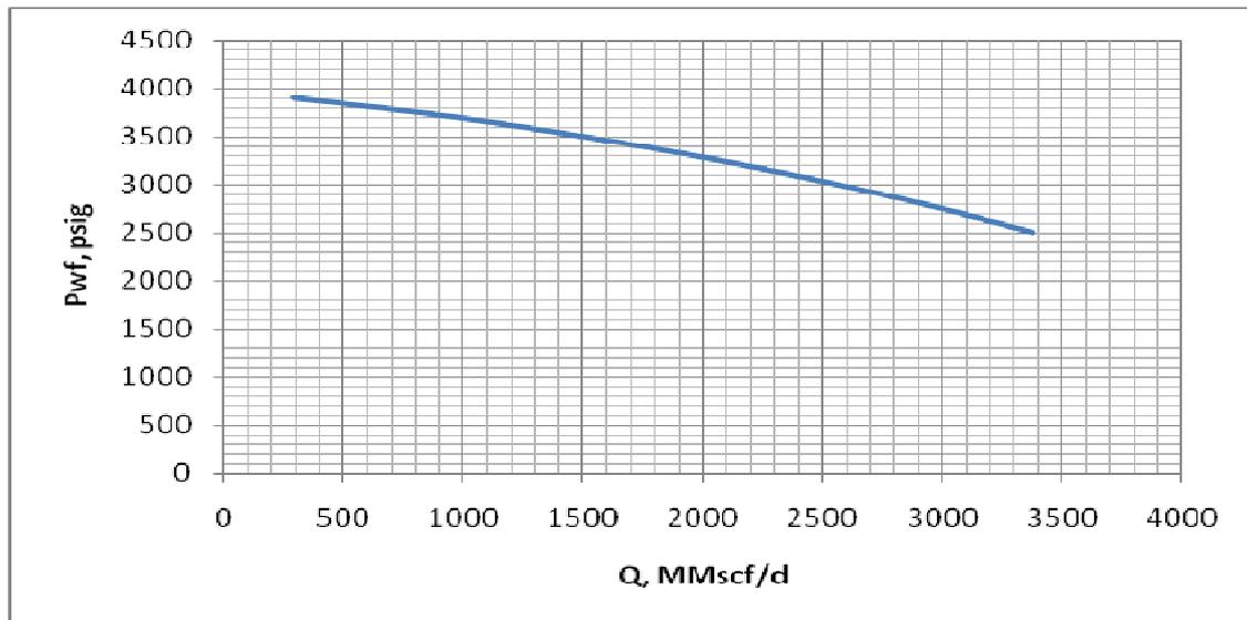
Fig. 3.3: A Plot of Well Flowing Pressure versus Deliverability
