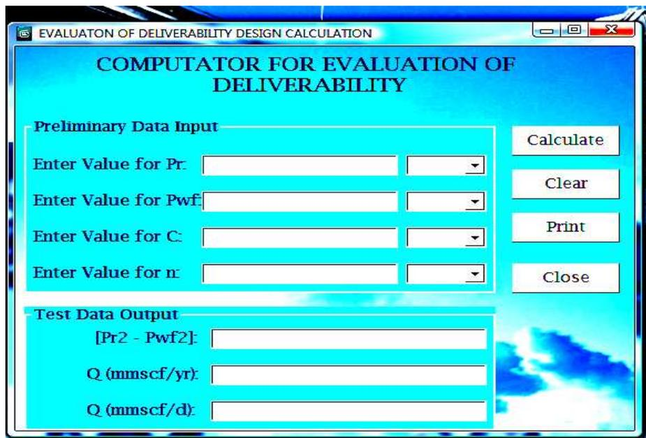
Fig 2.1: Program computator for evaluation of deliverability at given well flowing pressure
