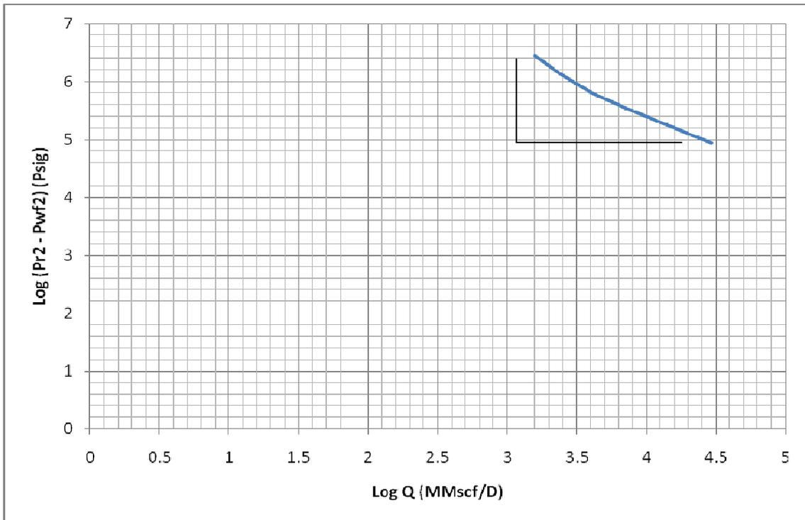
Fig. 3.1: Plot of Log  $[P_R^2 - P_{wf}^2]$  Vs. Log Q for the Depleted Oil Reservoir
