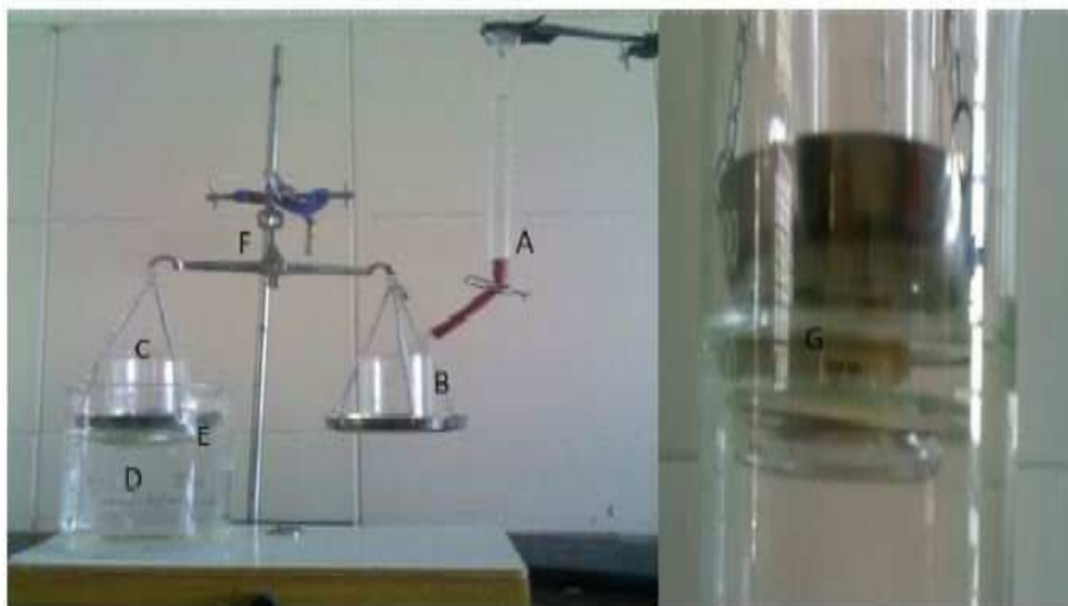
A: Burette B: Beaker for collection of water C: Wt. adjustment for pan D: 1 lit. Beaker having dissolution medium E: Glass slide along with mucous F: Modified physical double pan balance G: focus showing adherence of tablet to mucous membrane
