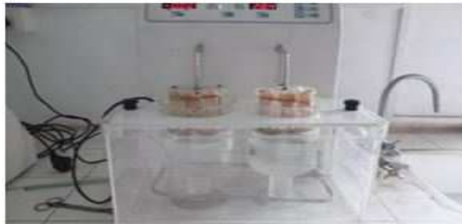
Fig: 10 Ex-Vivo Mucoadhesion test of Rebapimide mucoadhesive tablet
