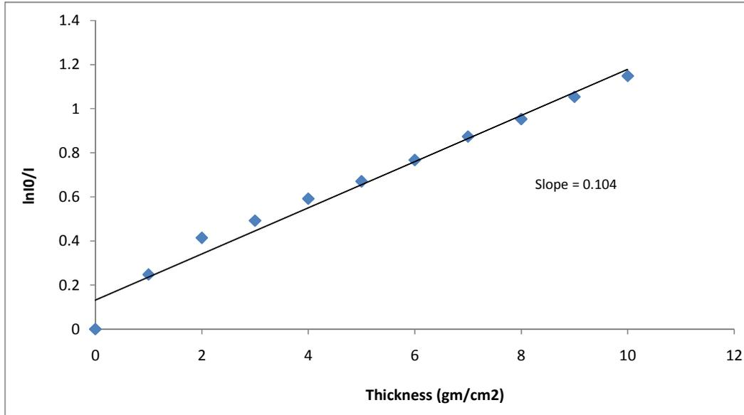
**Fig.1 Thickness in  $\text{gm}/\text{cm}^2$  vs.  $\ln I_0/I$  for zinc at 0.360 MeV.**
