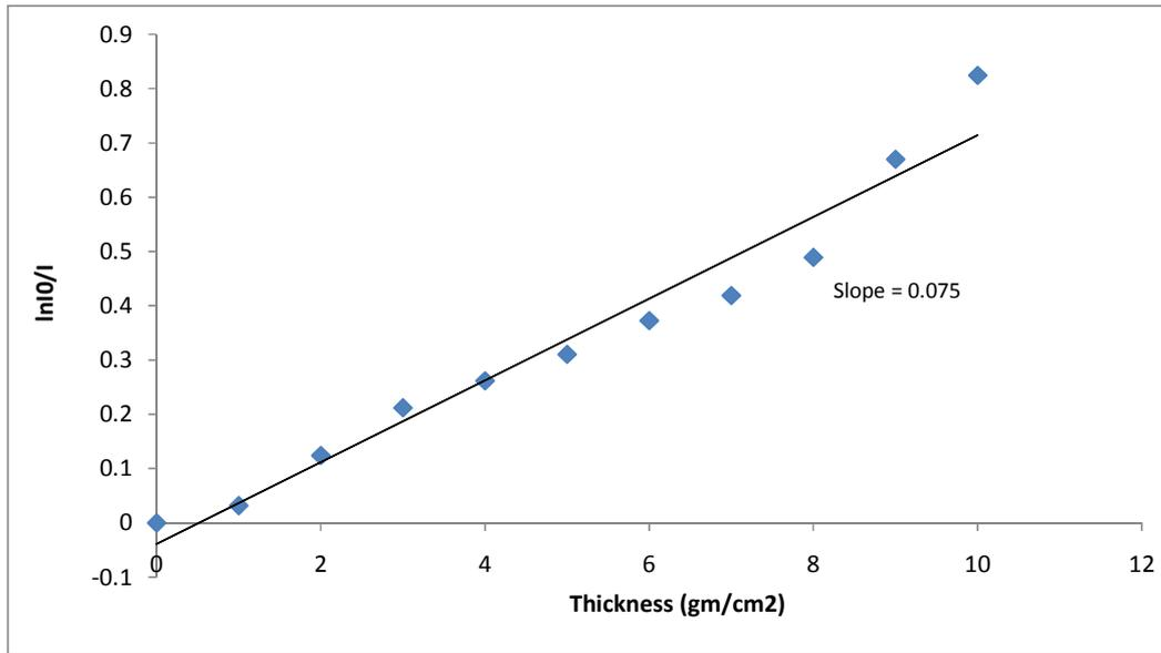
Fig.3 Thickness in gm/cm<sup>2</sup> vs.ln I<sub>0</sub>/I for zinc at 0.662 MeV.
