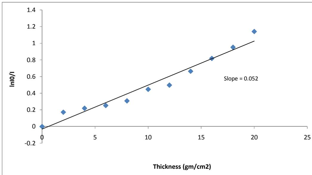
Fig.4 Thickness in gm/cm<sup>2</sup> vs.ln I<sub>0</sub>/I for zinc at 1.170 MeV.
