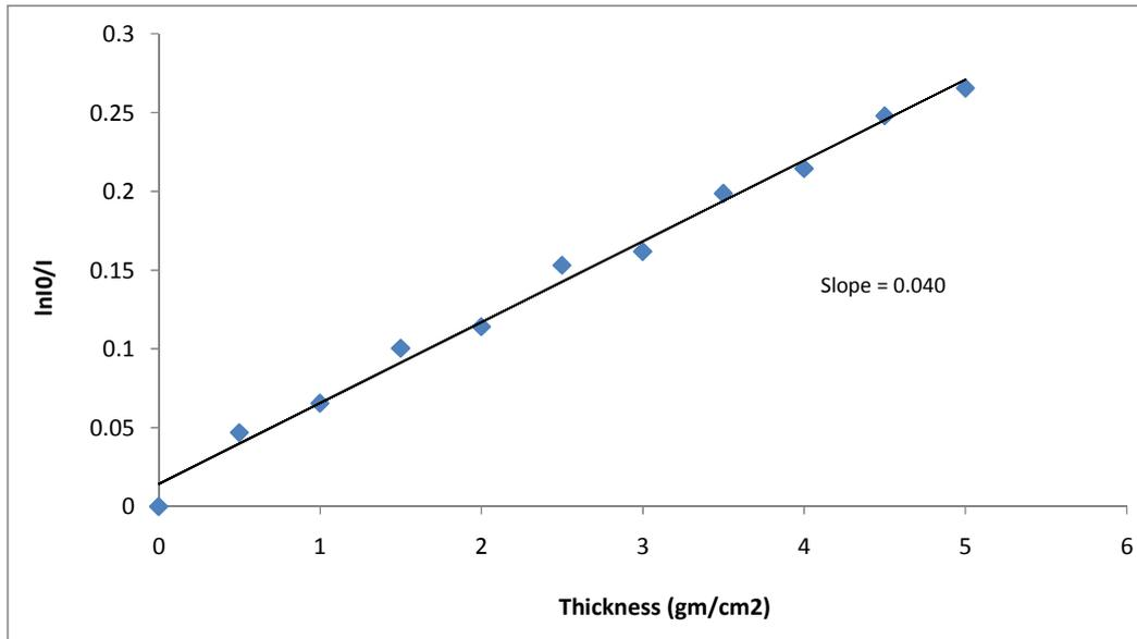
Fig.5 Thickness in gm/cm<sup>2</sup> vs. ln I<sub>0</sub>/I for zinc at 1.1280 MeV
