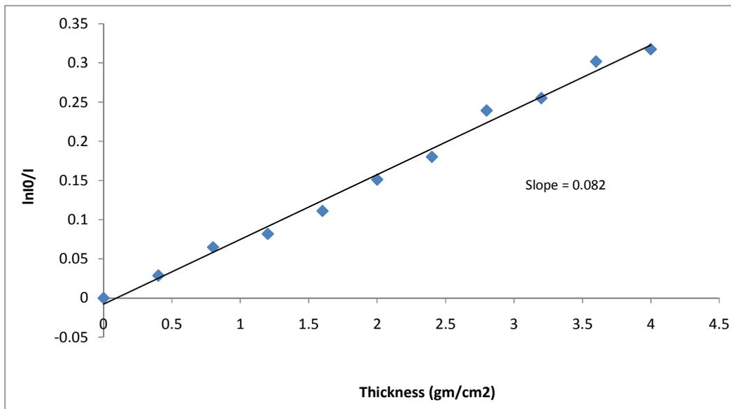
**Fig.2 Thickness in  $\text{gm}/\text{cm}^2$  vs.  $\ln I_0/I$  for zinc at 0.511 MeV.**
