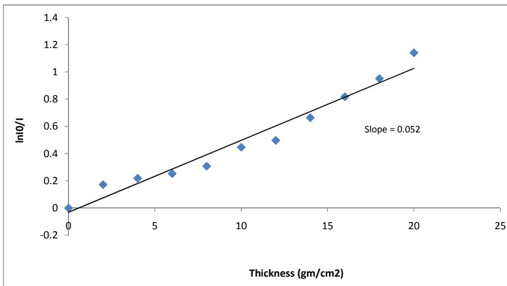
Fig.6 Thickness in gm/cm<sup>2</sup> vs. ln I<sub>0</sub>/I for zinc at 1.330 MeV.
