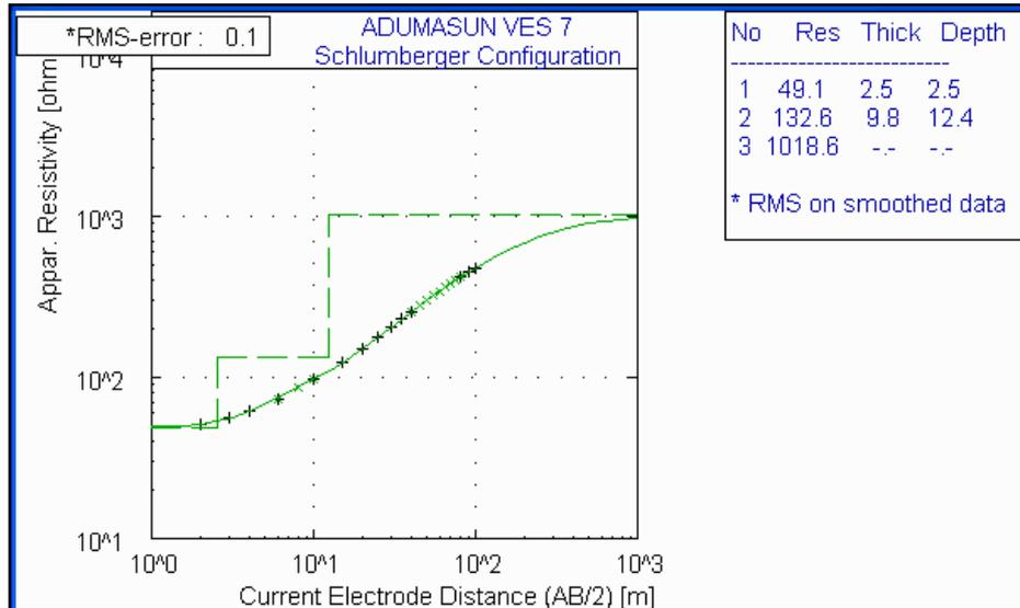
Figure 5(g): The modeled curve for VES 7.
