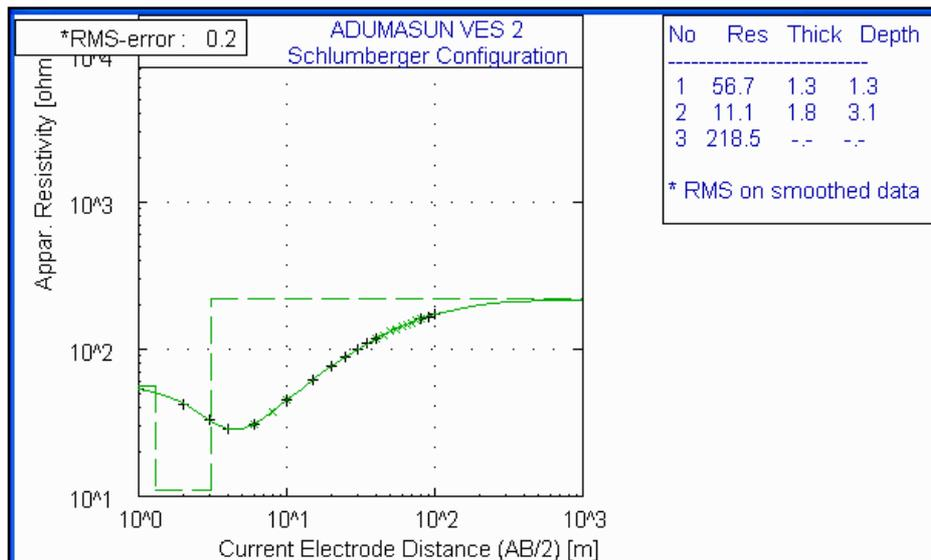
Figure 5(b): The modeled curve for VES 2.
