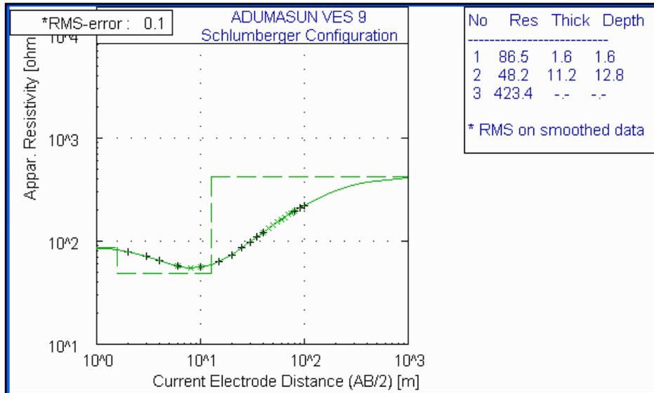
Figure 5(i): The modeled curve for VES 9.
