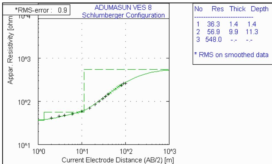
Figure 5(h): The modeled curve for VES 8.
