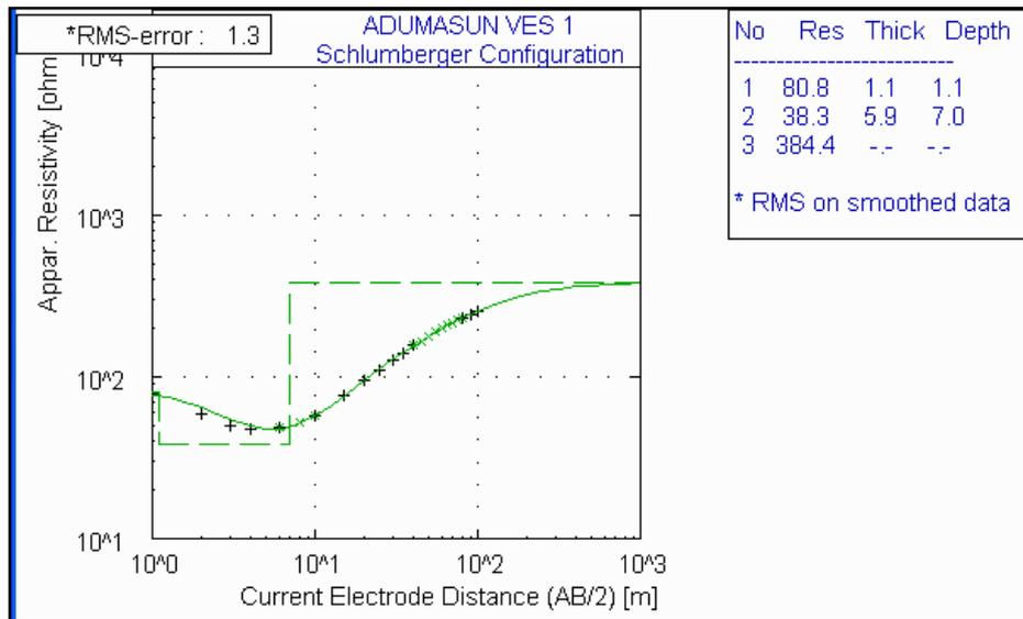
Figure 5(a): The modeled curve for VES 1.
