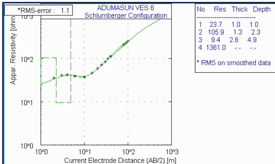
Figure 5(f): The modeled curve for VES 6.
