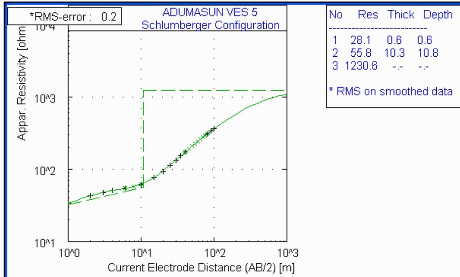
Figure 5(e): The modeled curve for VES 5.
