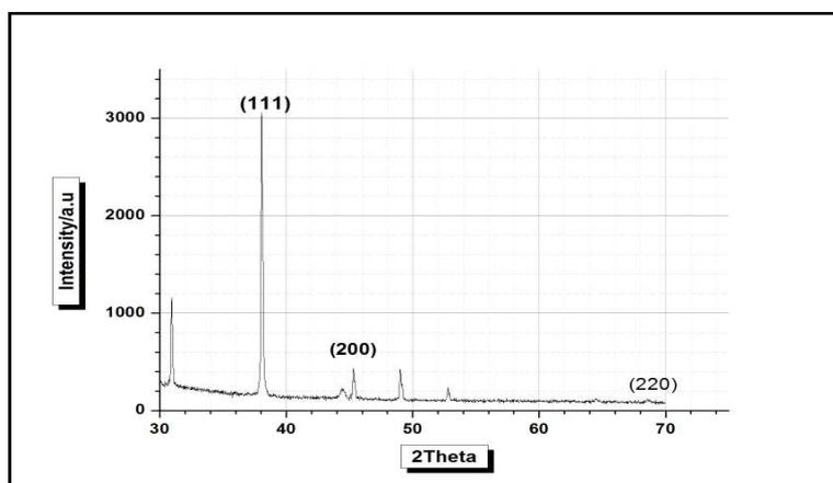
**Figure- 5:** X-ray diffraction pattern of gold nanoparticles biosynthesised using *Momordica Charantia*
