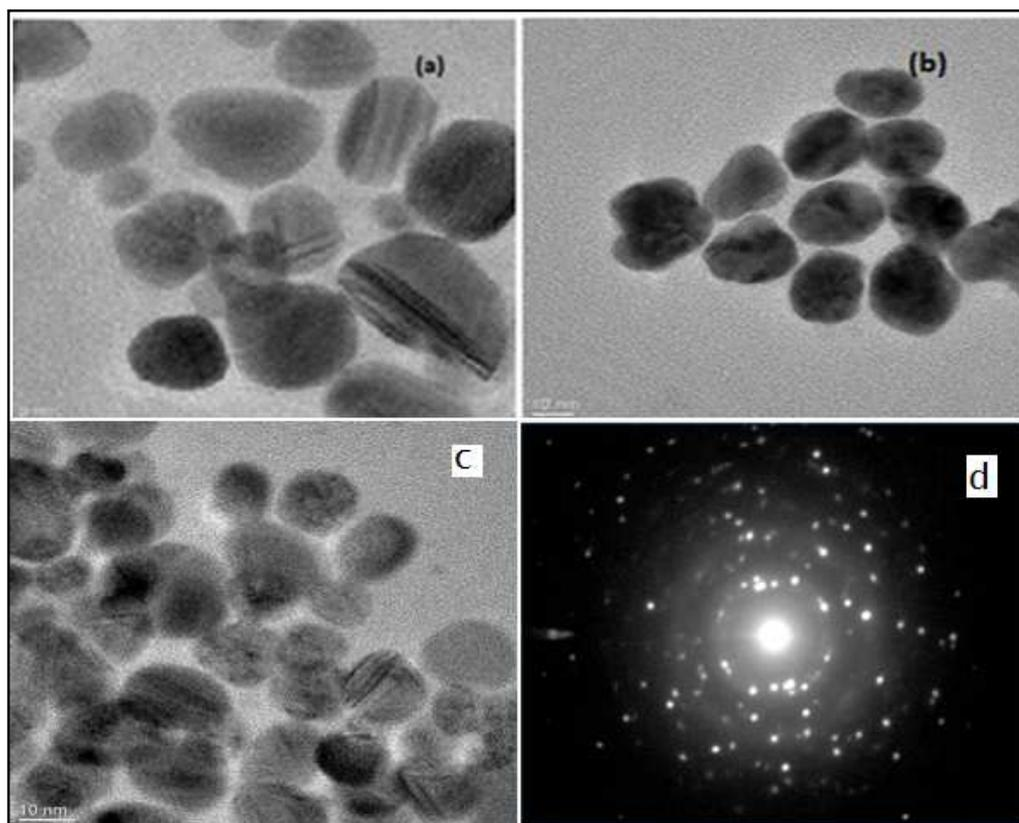
**Figure- 4:** HRTEM of GNPs synthesized using extracts of *M. charantia* at 30°C, pH 10 (b) 60°C, pH 10 and (c) 100°C, pH 10 and (d) The selective area energy dispersion (SAED) pattern showing that the nanoparticles are crystalline.
