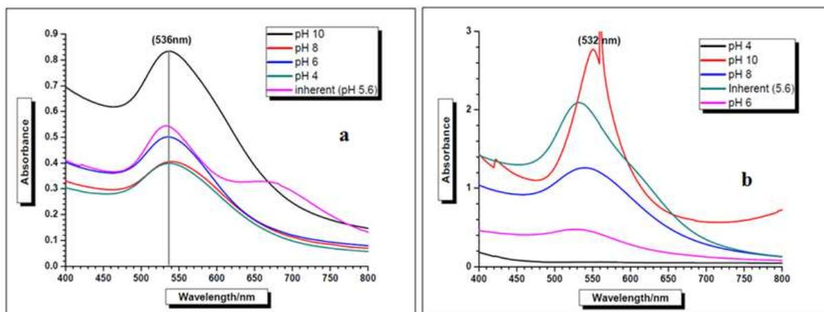
**Figure- 1: Impact of temperature and pH on synthesis on GNPs using extract of *M. charantia*; as recorded by the UV-Vis spectroscopy of the sample synthesized at (a) 30°C (b) 100°C.**
