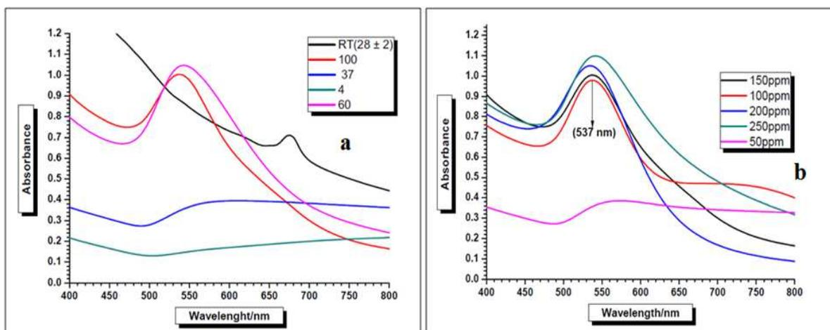
**Figure- 2: (a) Impact of temperature on synthesis of GNPs using extract of *M. charantia* at pH 10, 100 ppm aurochlorate; (b) Impact of aurochlorate concentration on synthesis of GNPs using extract of *M. charantia* at pH 10.**
