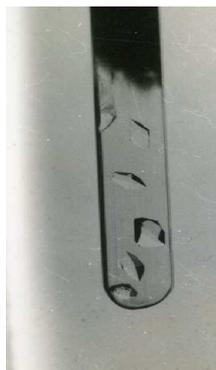
Fig. 2. Crystallization by gel method employing borosilicate glass tubes
