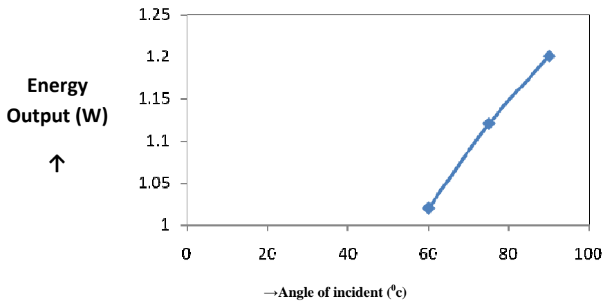
Fig.3.Variation of energy output (W) versus angle of inclination (°) for different values of angle of incident by considering height and discharge of water is 11 cm and 1100 cm³/sec.
