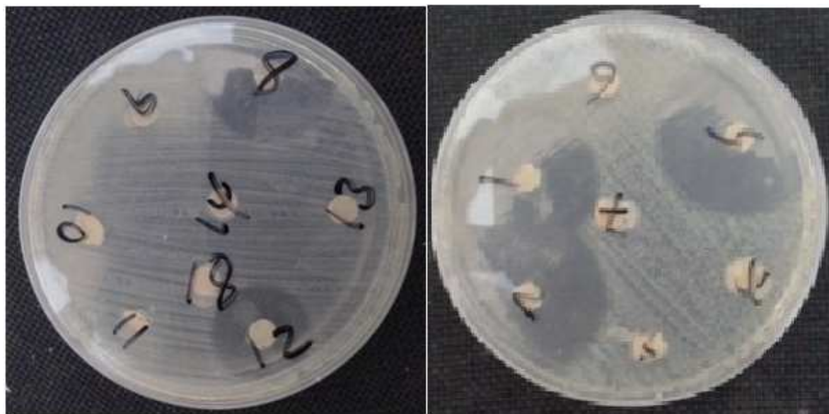
Figure-2: Disc diffusion test. Milk samples 1, 2, 5, 8, 12 showed inhibitory zone since they contained antibiotics
