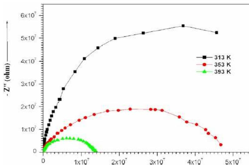
Figure 16: Cole-Cole Plot for ZnO NP doped PDLC
