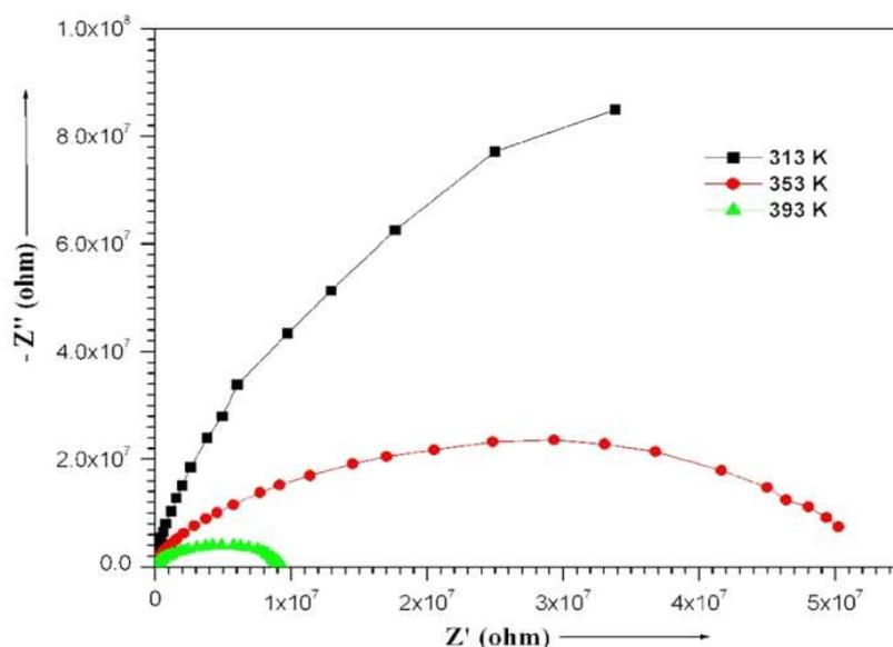
Figure 17: Cole-Cole Plot for CdO NP doped PDLC
