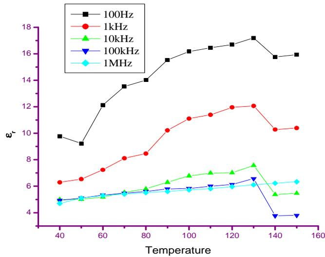
Figure 11 : Variation of dielectric constant with temperature for CdO doped PDLC for various frequencies.
