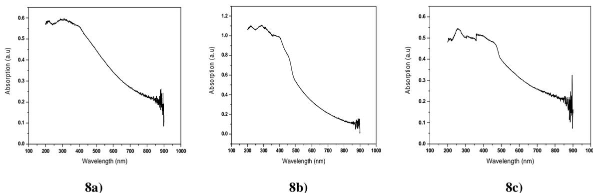
**Figure 8: Optical absorption spectrum (UV) for Pure PDLC and ZnO/CdO NP doped PDLC.**
