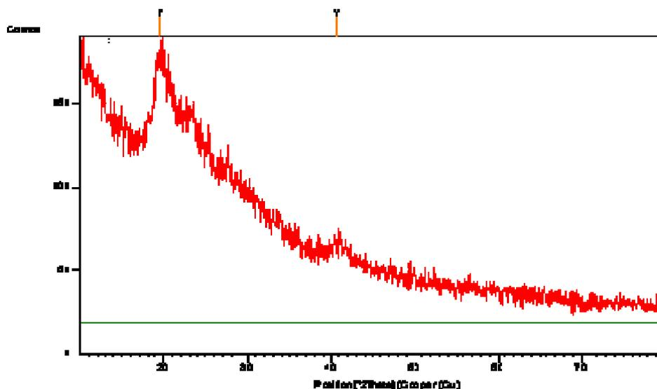
Figure: 2 XRD for the ZnO NP doped PDLC
