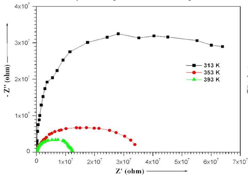
Figure 15: Cole-Cole Plot for pure PDLC
