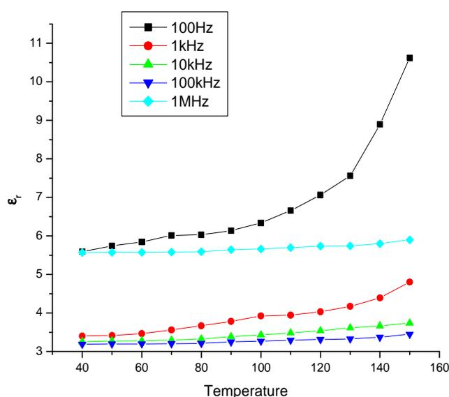
Figure 9 : Variation of dielectric constant with temperature for pure PDLC for various frequencies.
