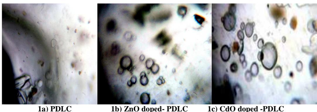
Figure: 1 Optical microscopy image for pure PDLC and ZnO/CdO NP Doped PDLC
