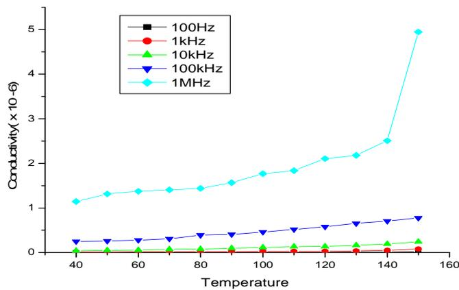
Figure 12 : Variation of AC conductivity with temperature for pure PDLC for various frequencies.
