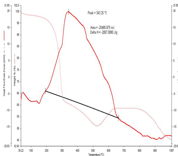
Figure 5: The TG/DTA for pure PDLC
