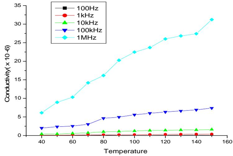
Figure 14 : Variation of AC conductivity with temperature for CdO doped PDLC for various frequencies.
