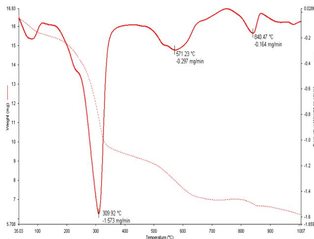
**Figure 7: The TG/DTA CdO NP doped PDLC**
