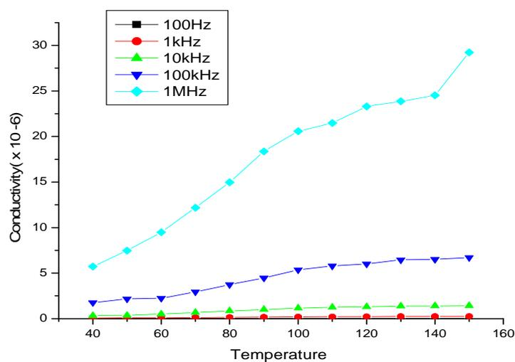
Figure 13 : Variation of AC conductivity with temperature for ZnO doped PDLC for various frequencies.
