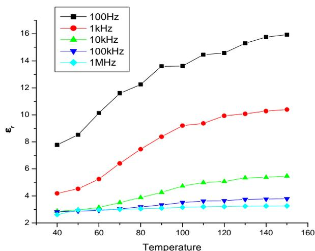
Figure 10 : Variation of dielectric constant with temperature for ZnO NP doped PDLC for various frequencies.
