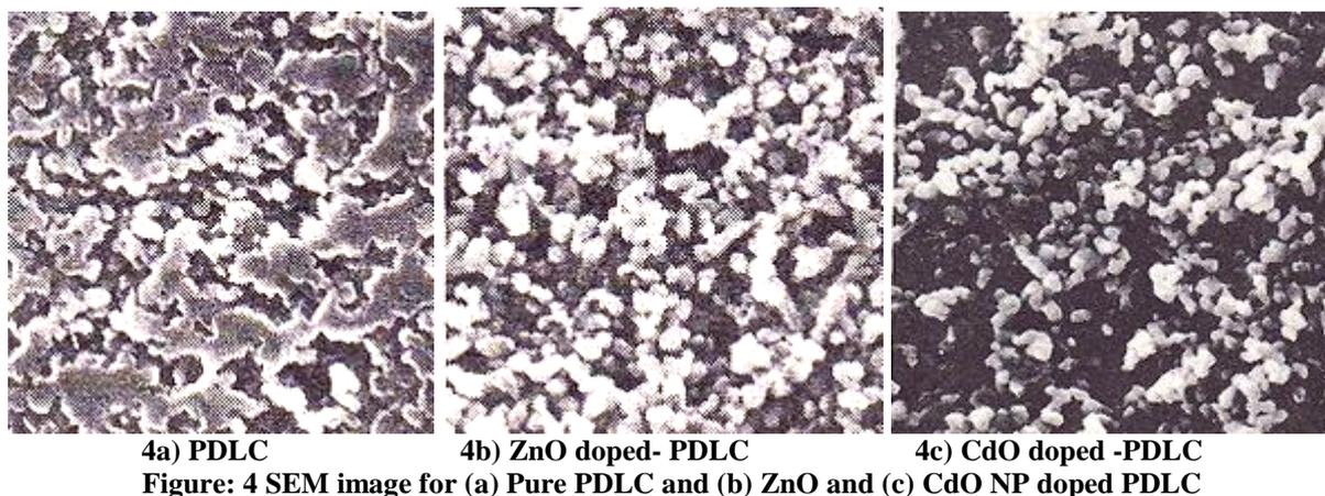
4a) PDLC                      4b) ZnO doped- PDLC                      4c) CdO doped -PDLC
