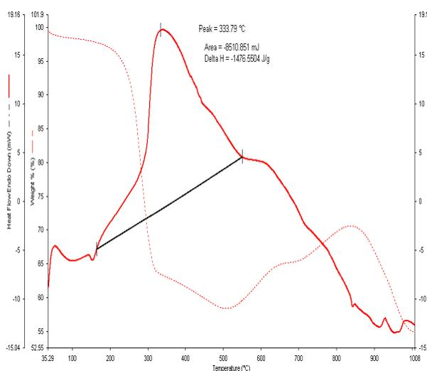
Figure 6: The TG/DTA ZnO NP doped PDLC
