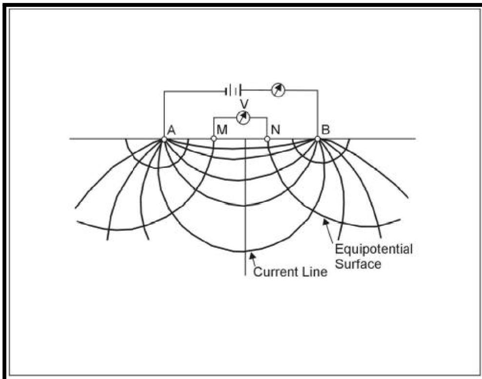
Figure2. Equipotentials and current lines for a pair of current electrodes A and B on a homogeneous half-space
