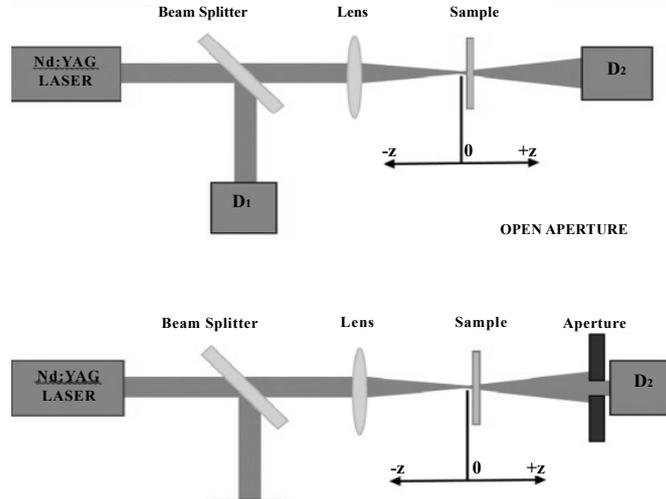
Figure 5: Experimental set for Z-scan technique
