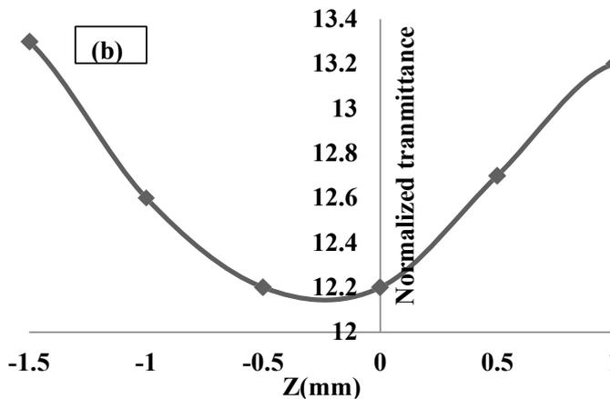
Figure 6b: The open aperture of Z-scan study for KHPMS crystal, respectively
