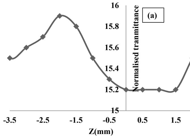
Figure 6a: The closed aperture of Z-scan study for KHPMS crystal, respectively
