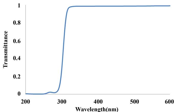
Figure 3: Transmission spectrum of the grown crystal KHPMS
