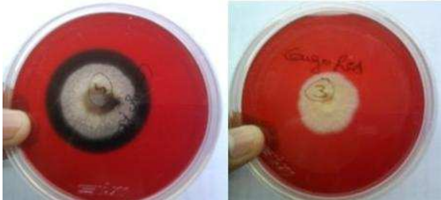
Figure 2: positive strain (left) of Aspergillus niger showing clearing zone, negative strain (right) of Aspergillus niger without any characteristic observation for CMCase activity.
