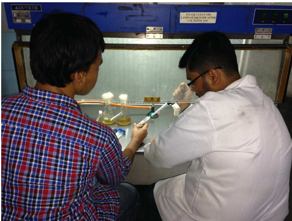
Fig 15: Preparation of broth with mixed oil samples and inoculums in a laminar flow
