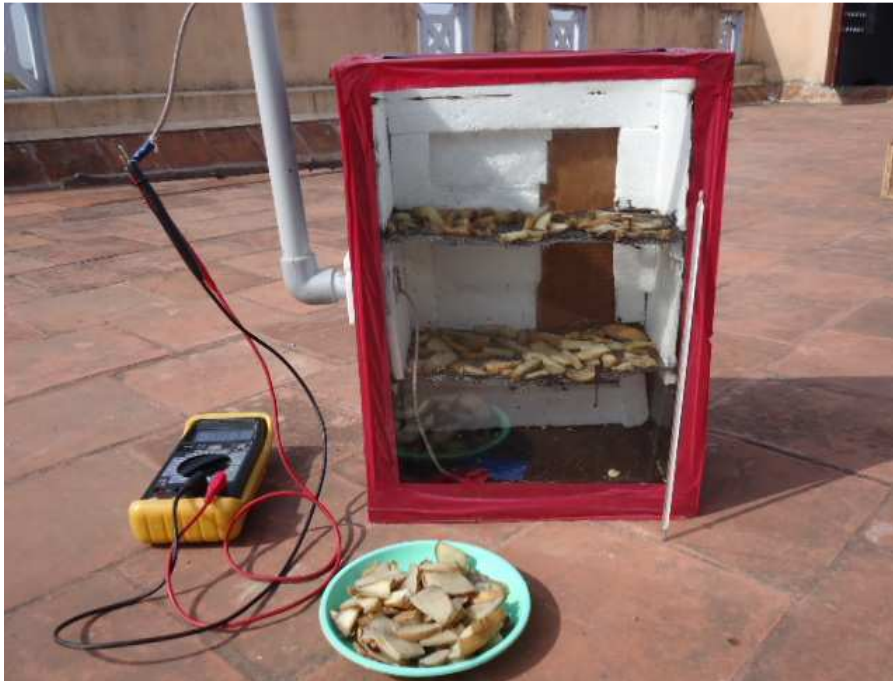
Fig.2 Experimental set up of box type solar dryer with potato slices
