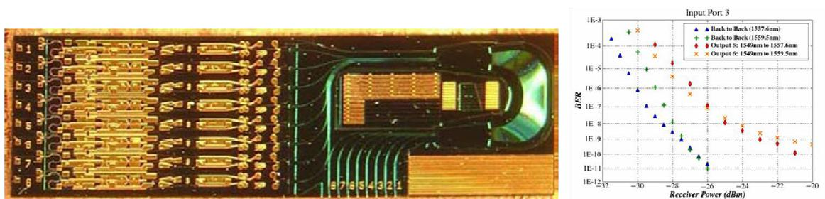
Figure 4 – Photograph of fabricated 8-channel MOTOR device; Bit error rate testing results, showing error-free operation at 40 Gbps
