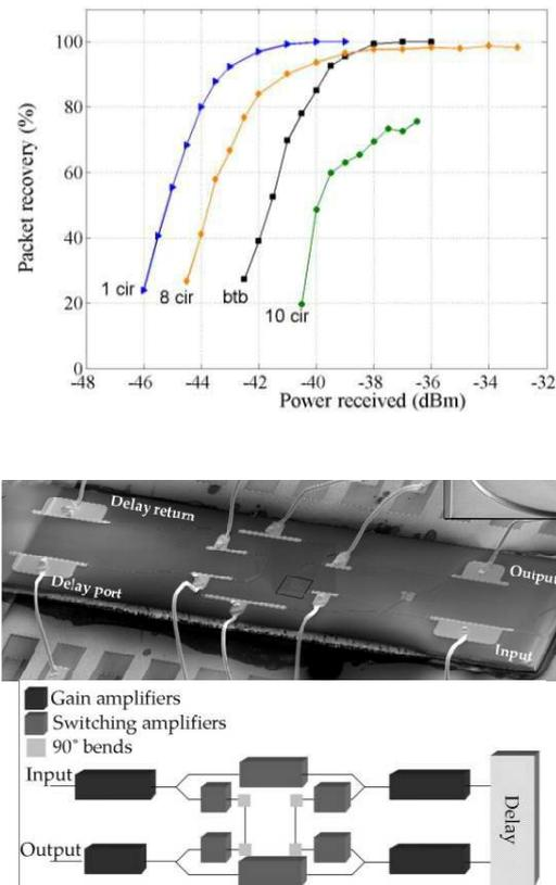
Figure 5 (top-left) Schematic of 2x2 switch with amplifiers (bottom left) SEM image of the switch affixed and wire-bonded to a submount (right) Packet recovery of 98% for up to 8 circulations (184 ns delay)
