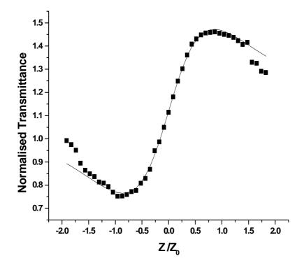
Figure.5 Measured z-scan of the dye victoria blue doped polymer film . The solid line is the calculated result with  $\Delta Ø_0 = 1.77$ .
