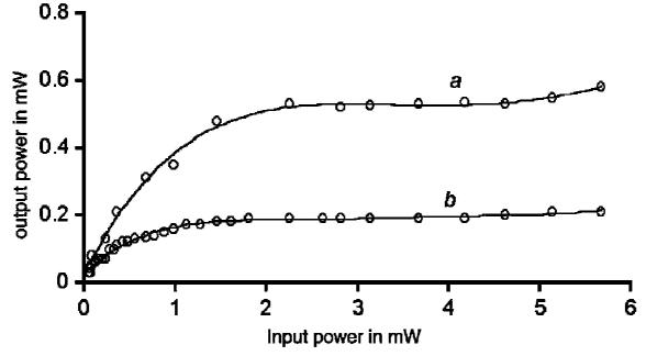
Figure.6 Optical Limiting of Victoria Blue in (a)nBA (b) in polymer thin film
