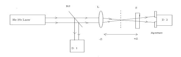
Figure.3 The closed z-scan set up. D1,D2 - detectors, BS beam splitter, L - convex lens, S- sample
