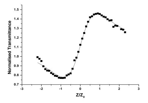
Figure.4 Measured z-scan of the dye victoria blue in nBA. The solid line is the calculated result with  $\Delta Ø_0 = 1.72$
