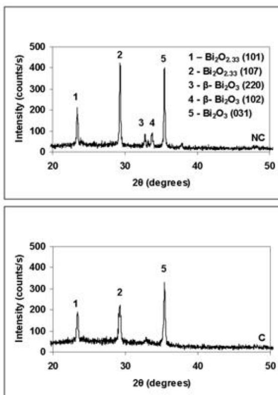
Figure 1 : XRD patterns of nonchopped (NC) and vapour chopped (C) bismuth oxide thin films oxidized at 573 K for 60 min. of thickness 150 nm.
