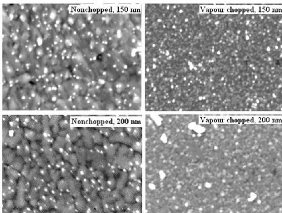
Figure 2: SEM images of 150 and 200 nm thick nonchopped and vapour chopped bismuth oxide thin films oxidized at 573 K for 60 min.
