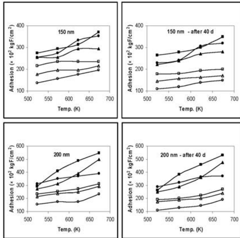
Figure 3: Adhesion as a function of oxidation temperature for as-prepared and aged nonchopped (hollow symbols) and vapour chopped (filled symbols) bismuth oxide thin films oxidized for (●, ○) 30, (■, □) 60 and (▲, △) 90 min.
