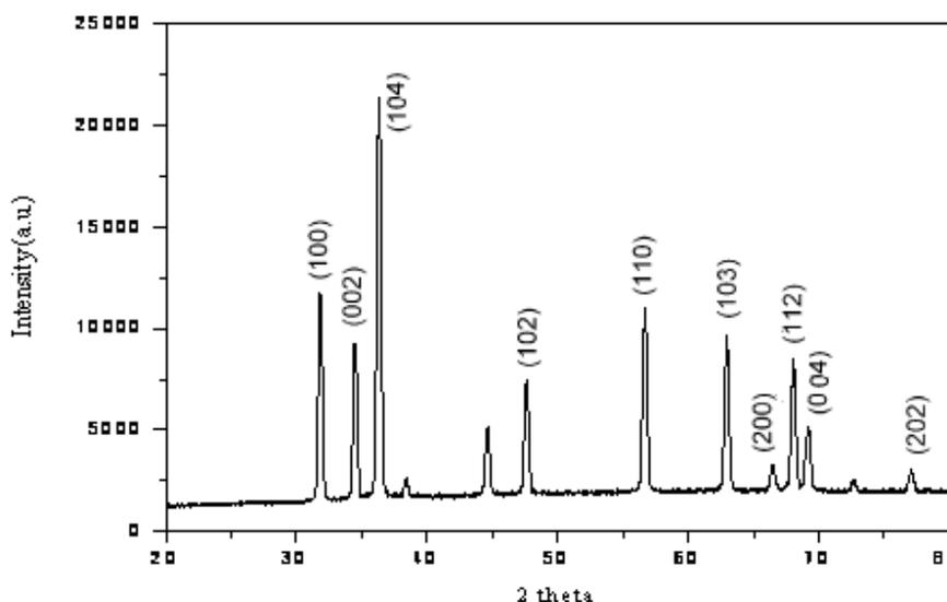
Fig.2. XRD pattern of ZnO nanoparticle
