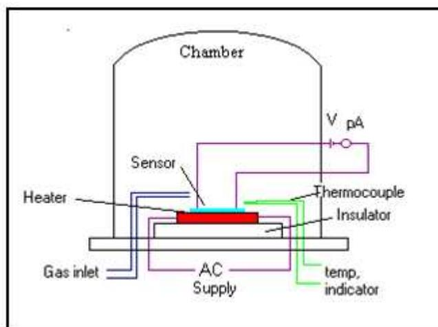
Fig.1. Block diagram of gas sensing unit
