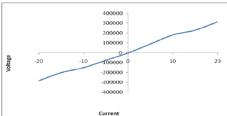
Fig.7. I-V Characteristics of the sensor
