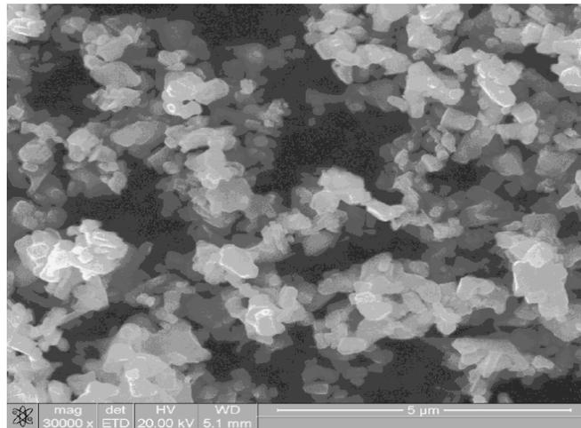
Fig.3. SEM image of ZnO nanoparticle
