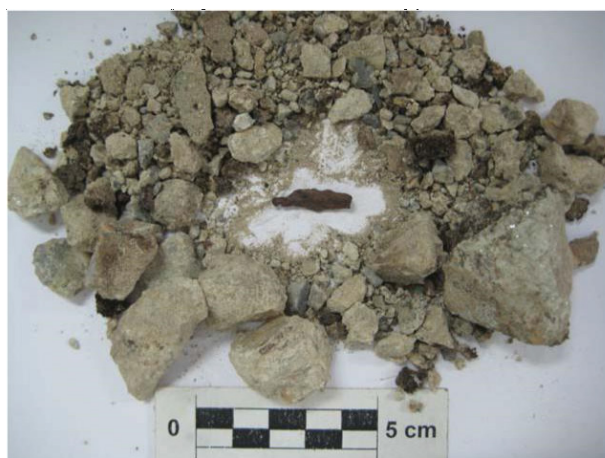
Figure 2: A sample of cyclopean concrete where the steel nail was found inside.
