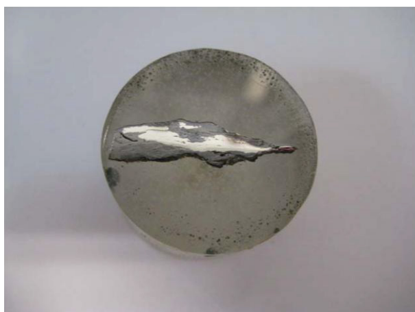
Figure 3: Steel nail found with traces of metalcore.
