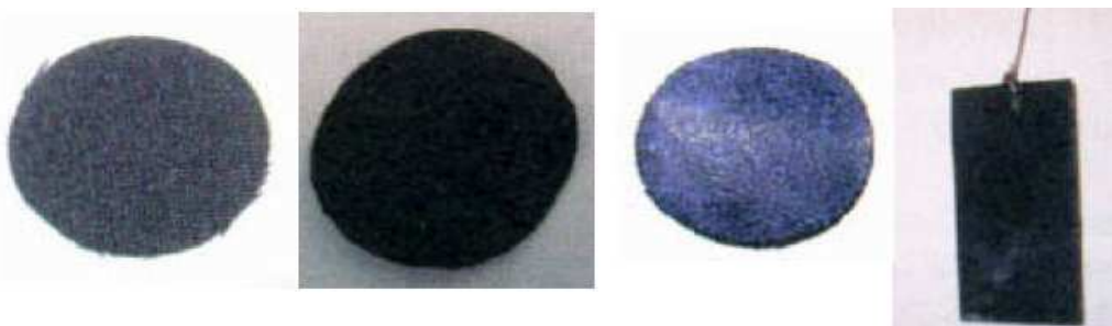
Figure.6. (a) Plain carbon cloth (b) carbon cloth coated with Pt catalyst on one side that typically faces the liquid (c) carbon cloth with a diffusion layer applied that typically faces the air (d) Square cathode used in two-chamber systems that is suspended in the water
