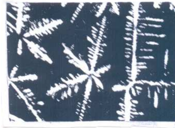
Fig. (c) Anisotropic growth of benzoic acid-camphor eutectic composite material at growth velocity 3 \times 10^{-7} \text{ m}^3\text{s}^{-1} ; magnification 100 x
