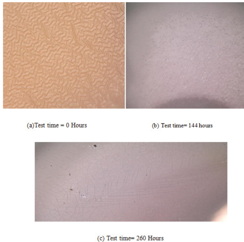
Figure 5: DLC surface topology variation with varying test time as indicated.
