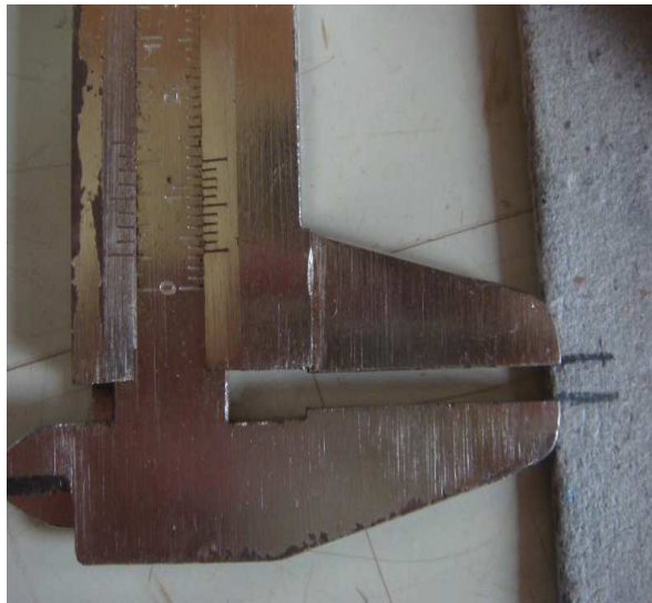
Fig.7 Measurement of ND by using vernier caliper in mm.
