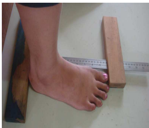
Fig.8 Measurement of foot length using custom made Brannock Device.
