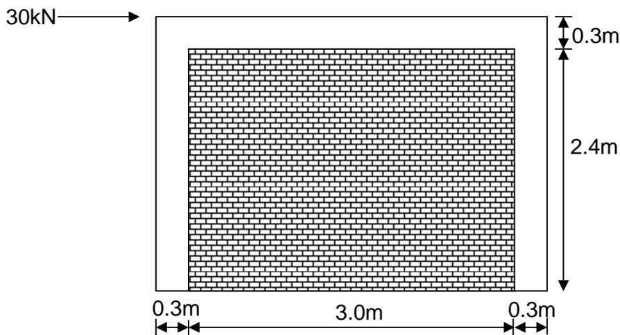
**Figure 3: Infilled reinforced concrete frame structure under the action of a static horizontal load**
