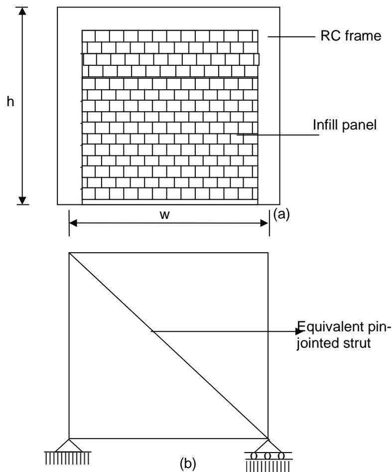
Figure 1: (a) infilled reinforced concrete frame (b) equivalent one-strut, macro-model
