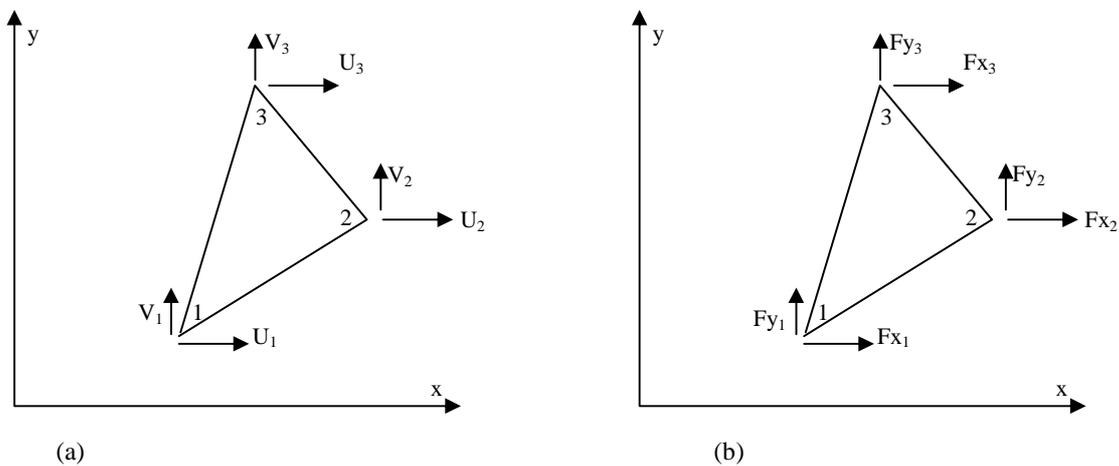
Figure 2: (a) Nodal displacements vector (b) Nodal force vectors, displayed in the Cartesian co-ordinate system.
