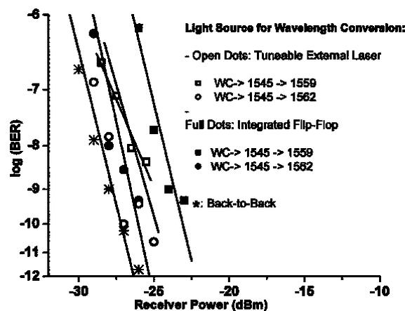
Fig. 5. BER measurements for static flip-flop operation.
