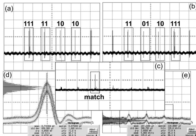
Fig. 4. Experimental results of label processor (a) incoming labels, (b) local labels, (c) match pulse, and (d), (e) show corresponding “1” and “0” levels.
