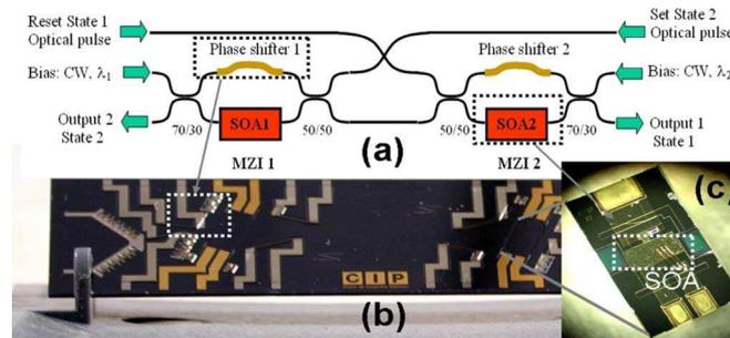
Fig. 2. Developed flip-flop using hybrid technology: (a) schematic of device, (b) planar silica motherboard, (c) daughterboard with twin SOAs flip chipped and wirebonded.
