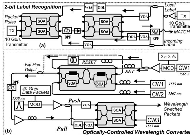
Fig. 3. Experimental setups of the all-optical network systems, (a) all-optical label processor and (b) optically controlled wavelength converter.
