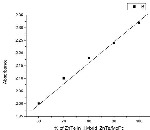
Fig:5 Variation of absorbance with conc (60, 70,80,90,and 100mg) of ZnTe in Hybrid ZnTe/MgPc.
