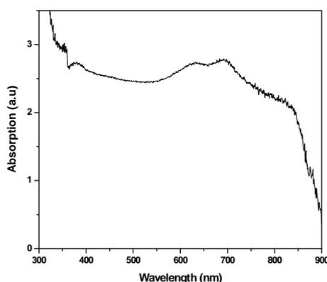
**Fig:4** Absorption spectra of Hybrid ZnTe/MgPc air annealed at 150°C.
