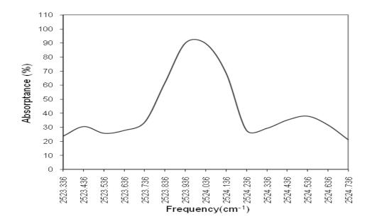
Figure 2: Absorptance of a 4  $\mu$ m free electron laser beam for a 0.1 atm-cm path length of SO<sub>2</sub>.
