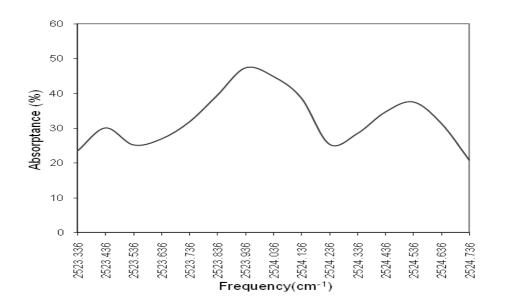
Figure 1: Absorptance of a 4  $\mu$ m free electron laser beam for a 0.01 atm-cm path length of SO<sub>2</sub>.
