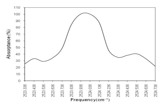
Figure 3: Absorptance of a 4  $\mu$ m free electron laser beam for a 1 atm-cm path length of SO<sub>2</sub>.
