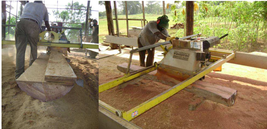
Figure 5: Milling of Cylicodiscus gabunensis (left) and Manilkara multinervis (right) logs with a Forestor swivel saw machine
