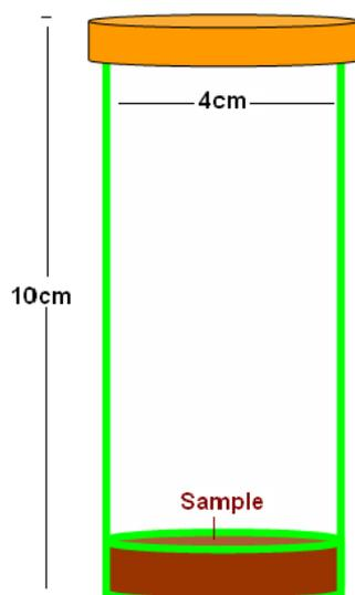
Figure-1. Schematic diagram showing the geometry of the CR39 and LR115-II Solid state Nuclear Track Detectors based radon passive dosimeter.
