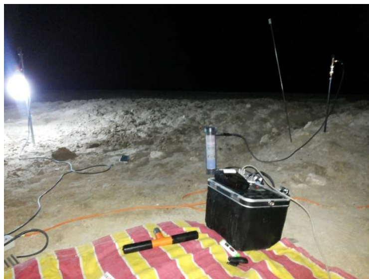
Figure 4 Active methods for measuring radon concentration in soil
