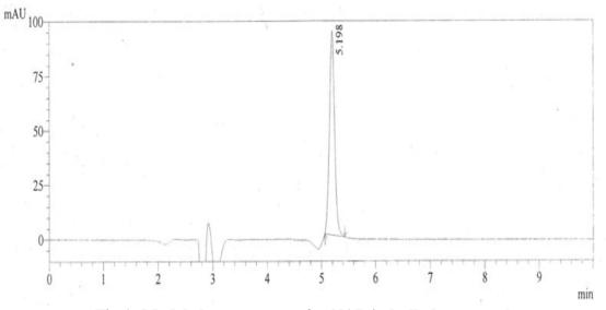
Fig 1: Model chromatogram for NAL in bulk drug sample
