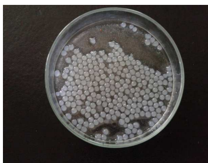
Fig 3: Immobilized Enzyme in gel beads
