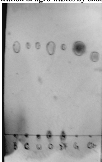
Figure 5. Thin layer chromatographic analysis of the end products of saccharification of the agro wastes by endoglucanase of R.oryzae .
