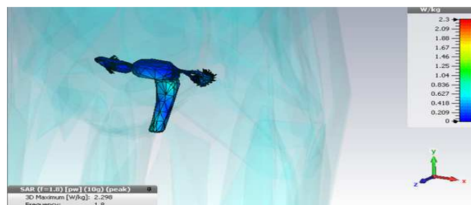
Figure 37: effect of radiation with frequency of 1.8 GHz on female ovary in distance of 2 meter from source
