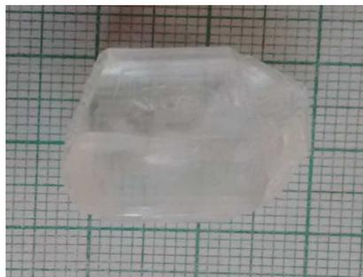
Fig 2(b). Photograph of as grown Zinc doped LAHC monohydrate
