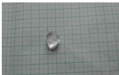
Fig1. Photograph of as grown Pure LAHC monohydrate crystal
