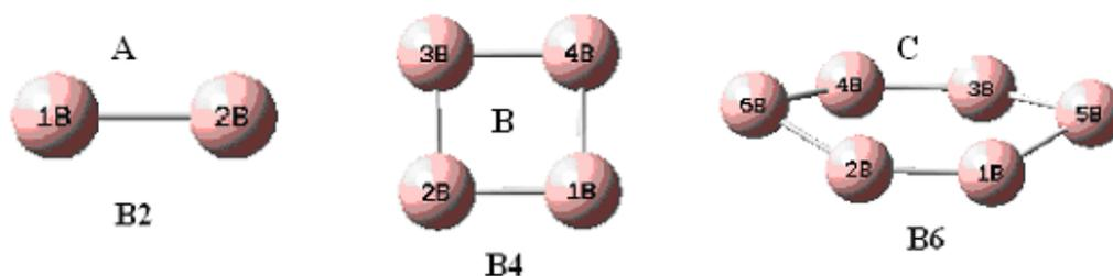
FIG-1 Optimized structures of Boron Clusters
