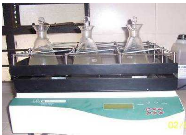
Plate No.4 Raw water sample treated with M. oleifera seed powder and kept on the shaker for 30 min at 110-120 rpm.
