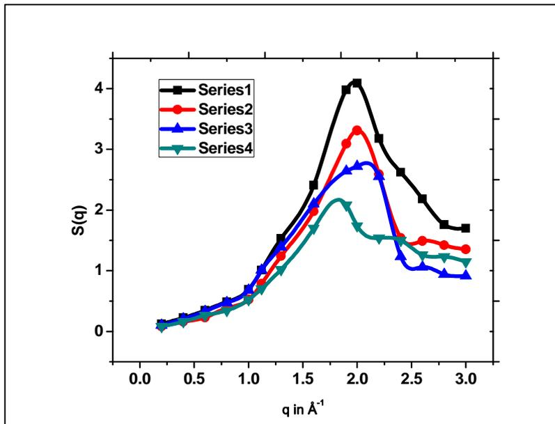
Fig2: Variation of  $S(q)$  with  $q$  at  $T=0.6\text{K}$ . Series 1 and 2 are for the Gaussian equivalent of Lennard Jones potential and series 3 and 4 are for hardcore followed by square well type of potential for  $m^*/m=1.6$  and  $2.0$  respectively.
