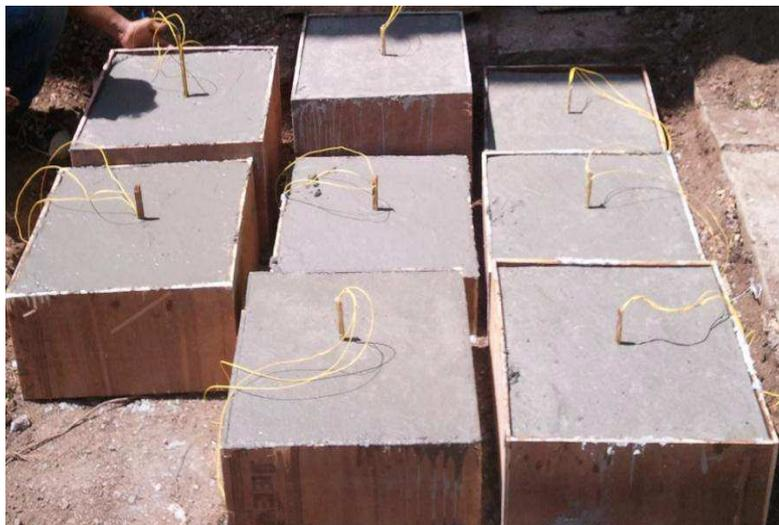
**Fig.2. Concrete slabs with thermocouple**
