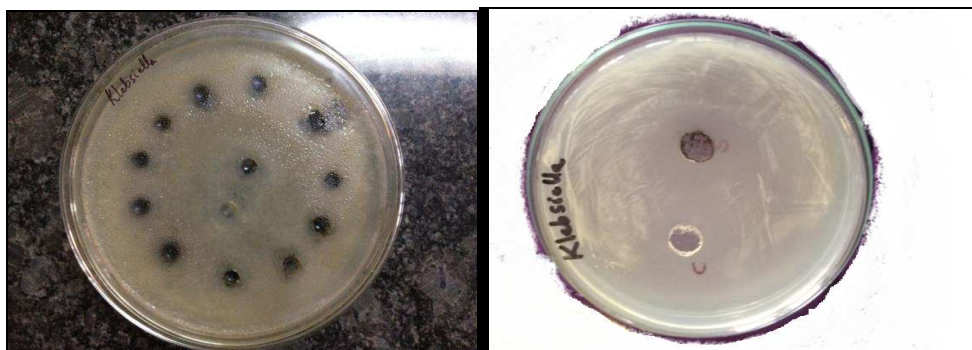
Figure 7. Photographic image of zones of inhibition at various concentrations of PANI on Staphylococcus sps and Klebsiella sps
