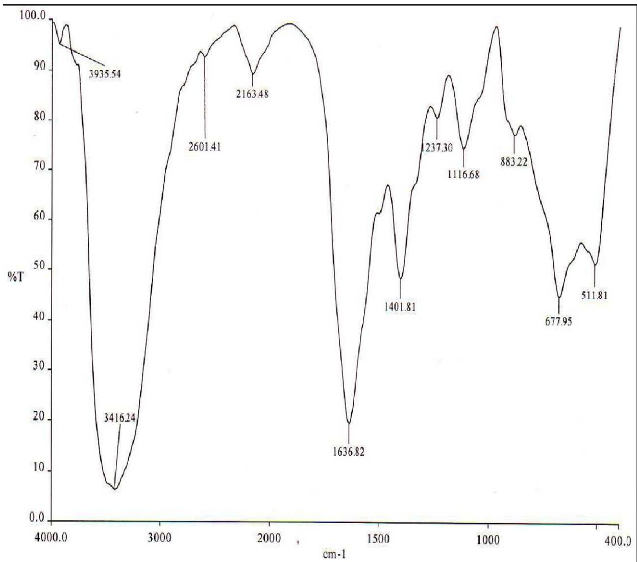
Fig.2. FTIR spectrum of TGZC crystals
