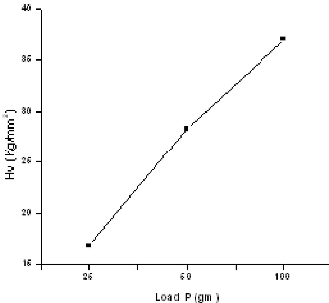
Fig.3. Microhardness Curves of TGZC crystals
