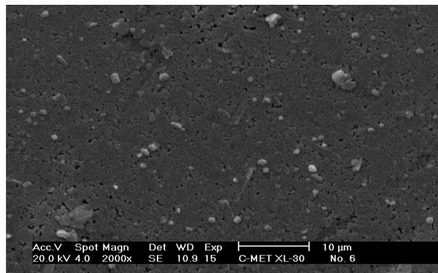
Fig. 7 SEM micrograph thin film of Zn-doped PbI<sub>2</sub> (2000Å)
