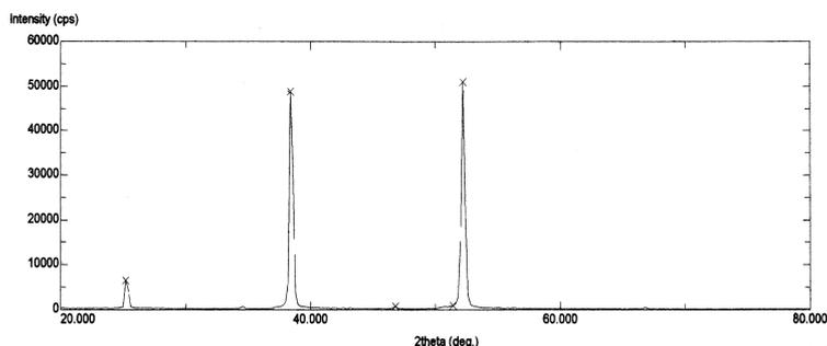
**Fig. 2 X-ray diffractogram for Cu-doped PbI<sub>2</sub> thin film (4000Å)**
