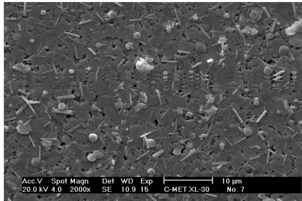
Fig. 6 SEM micrograph thin film of Al-doped PbI<sub>2</sub> (2000Å)
