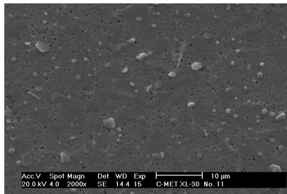
Fig. 4 SEM micrograph thin film of Cu-doped PbI<sub>2</sub> (2000Å)
