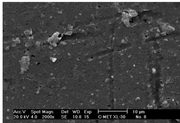
Fig. 5 SEM micrograph thin film of Cu-doped PbI<sub>2</sub> (4000Å)
