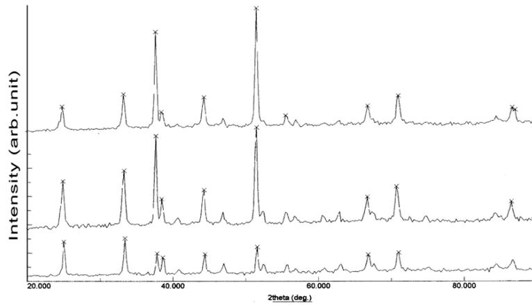
Fig. 3 X-ray diffractogram of Al-doped PbI<sub>2</sub> (From top 0.1M, 0.5M & 1M respectively)
