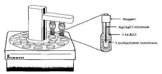
Fig. 3: Commercially sold taste-sensing system (SA402BJ Intelligent Sensor Technology, Inc.).
