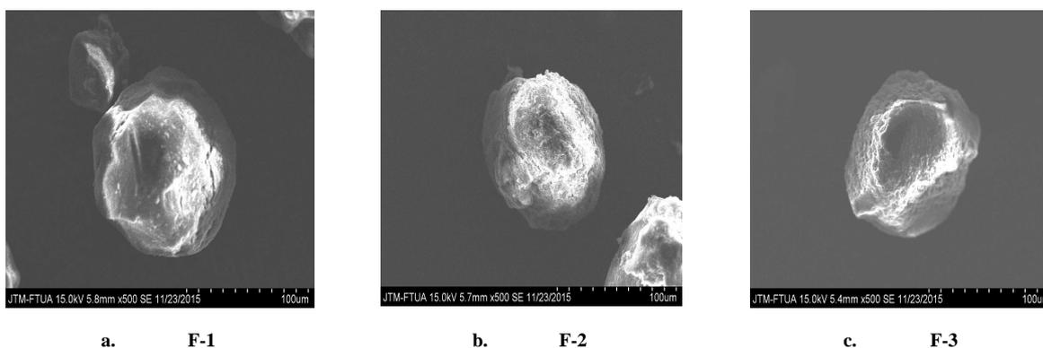
Figure 3. Scanning Electron Microscopy of microspheres F1 (Formula 1), F2 (Formula 2) and F3 (Formula )
