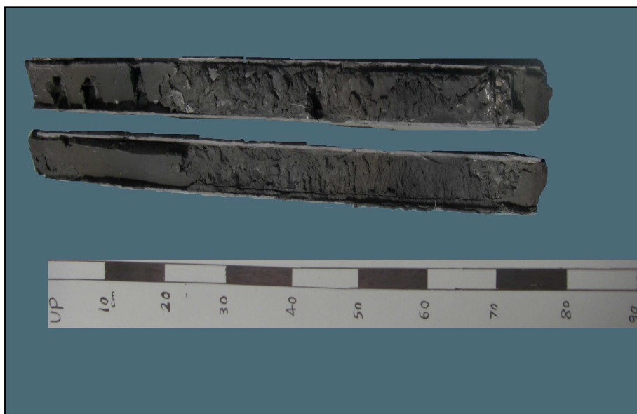
Figure 2: Exposed core samples in the sampling pipe removed from lagoon sediments
