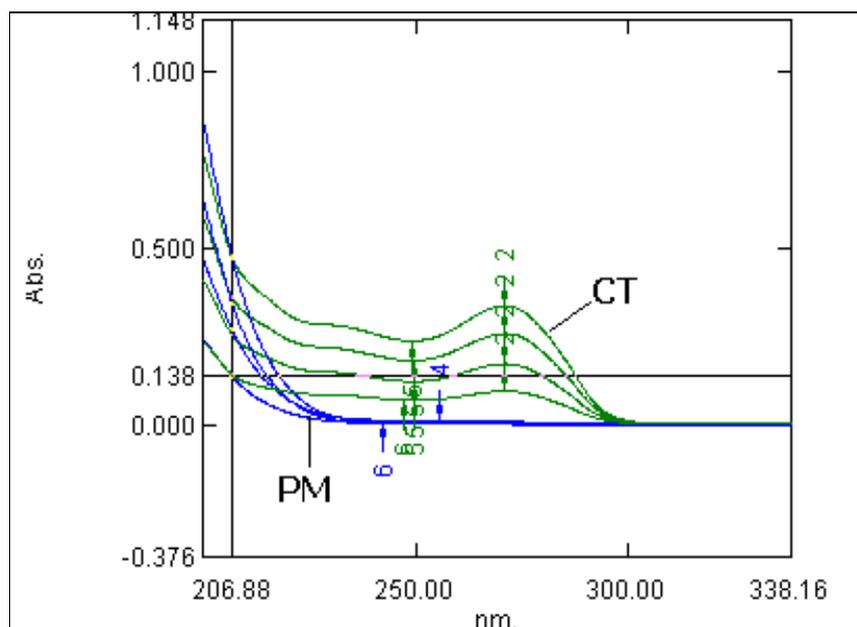
Figure: 2 Overlay Normal Spectra of CT and PM in distilled water
