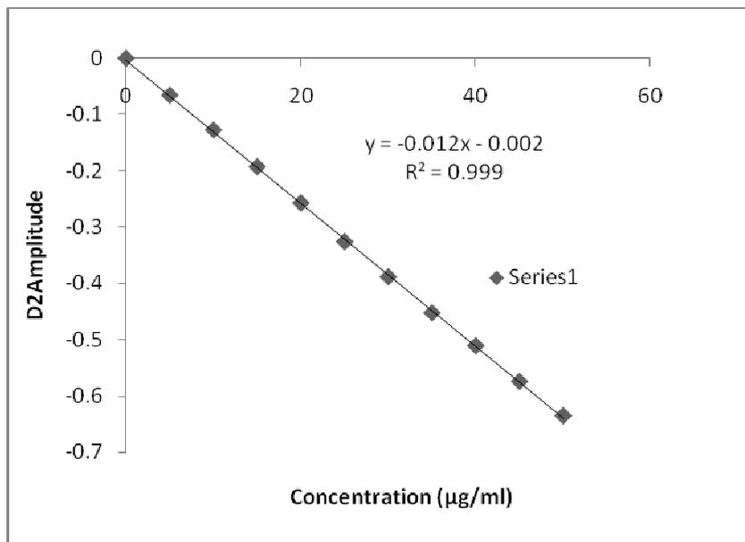
Figure: 3 Calibration Curve of CT (5-50 $\mu\text{g/ml}$ ) at 274.60 nm
