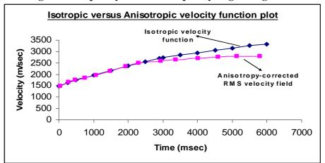
Fig. 8: Final isotropic and anisotropy-corrected velocity functions at a CDP location along the survey
