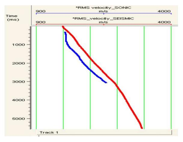
Fig. 5: Sonic (blue) and Seismically (red) derived RMS velocity fields
