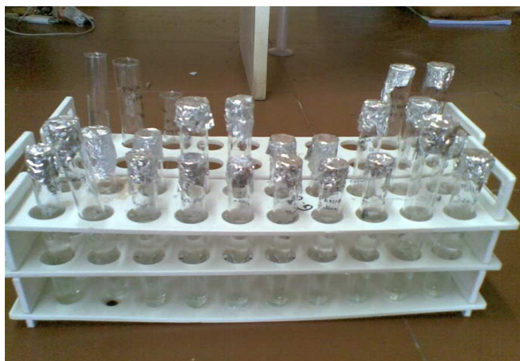
Figure 2: Test tubes containing inverted durham tubes for MPN analysis
