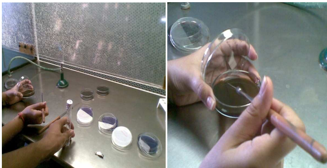
Figure 3 and 4: Macconkey agar and EMB agar plates being inoculated with water samples
